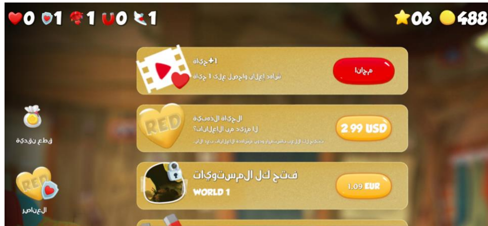
Figure 3 - An example of a game which is not "internationalized" the developers did not create the textboxes to handle the Arabic script and therefor the translated text turns into unreadable gibberish.
